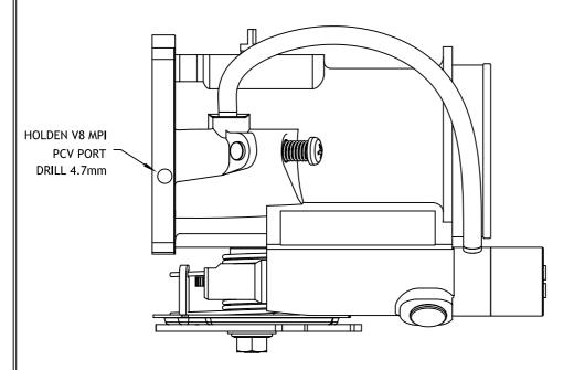
The GASRESEARCH Gold Series Throttle Bodies come with partially drilled holes to accommodate vacuum advance, evaporative emission, and vapour injection lines. These holes must be drilled through as required by each application. We recommend that the vacuum advance line only be used with regraphed distributors.
